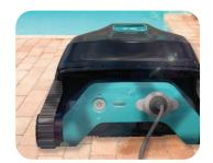
Inductive Charging Magnetic Connect for super easy snap-in-place charging
