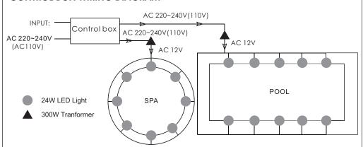
⚠ Warning: load of the control box should not exceed 2\*300W.
