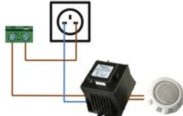
Connection: Device power < 2A (230V, 500W, 120V 250W)
