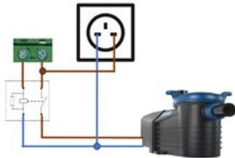
Connection: Device power < 2A (230V, 500W, 120V 250W)
