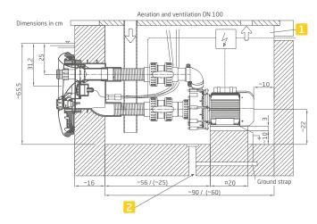
Sufficiently dimensioned drain required
