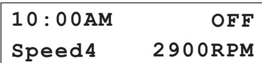
During power up: time, pump status, speed setting will be displayed on the screen.
