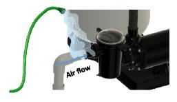
3. Piping Valve connection leakage. Check the union (fitting) between the pool pump and the valves. It is a pretty high chance for missteps when take pump apart.
