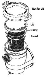
2. The strainer transparent lid is not tight. Oring has been damaged. The nut for lid will be damage if harmer is applied for tighten. Basket is not seat in the proper position
