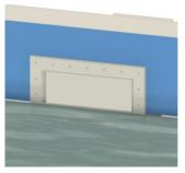
1. The level of the pool water is too low and doesn't cover enough to the skimmer. It is recommended to keep the water halfway to three-quarters up the skimmer.
