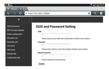
Type SSID name and password, repeat the same password, then press "Submit". The EPV Wi-Fi SSID and password is changed and you need to re-connect the EVP Variable speed pump Wi-Fi by new assigned SSID and Password. Scan QR code or type IP address 192.168.8.1 to access the web server page again.
