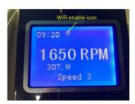
If there is no Wi-Fi icon display , press the "MENU" button and roll down to items 10 by "▼" , press " ENTER to access Wi-Fi setting.
