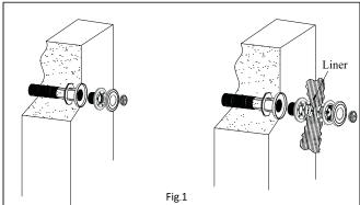
The suction nozzles can be assembled with threaded wall conduit 2" or assembly the connections  $\varnothing$ . 50 mm with PVC glue.
