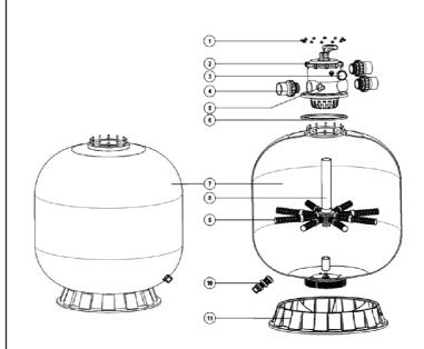
Notes:9\* 01172010 Laterals (185mm) for V700B 9\* 01172011 Laterals (233mm) for V800 & V900 9\* 89010613 Laterals (129mm & 185mm) for V1000 9\* 89010614 Laterals (129mm & 233mm) for V1200
