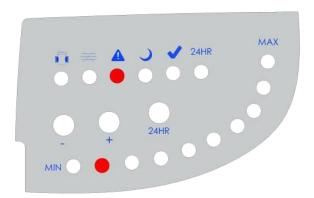
Case 3. salt level <4000ppm , calcium deposit on the cell or cell's water level too low.
