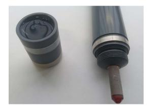
3) Caution: Before screwing again the header cap to the sensor body, the silicone ring must be removed, uncovering the small hole shown in the following picture:
