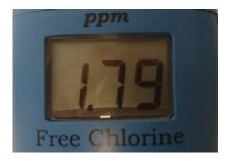
b. Chlorine Menu -> Select "calibration" and press OK. Wait until the reading is stable:
