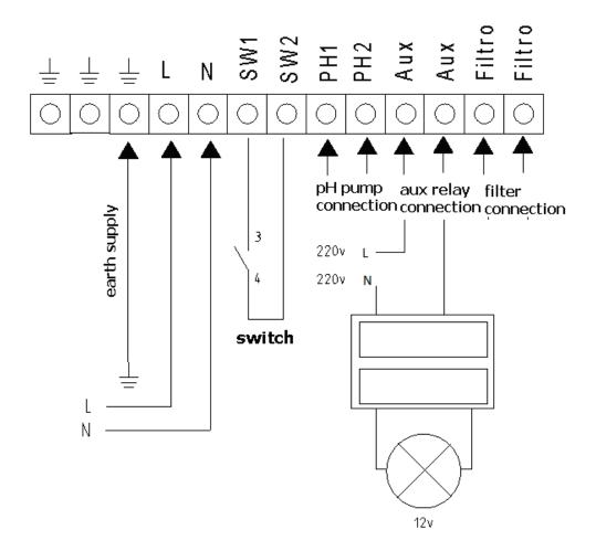
Attention: Never exceed 12A when using the auxiliary relay. For higher currents, supplement the circuit with a contactor.
