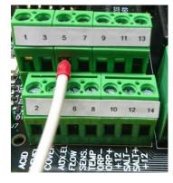
b) Flow Switch: Connect the two cables from the switch to the inputs 5 and 6. If this system is used, just let the white cable from the cell
