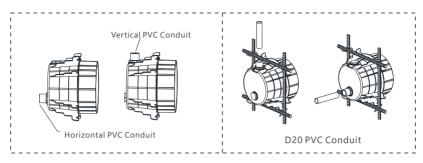
2. The niche and the concrete wall should be seal 3. Lead the power cord with connector through with sealant to prevent water get inside. the niche
