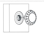
4. Screw light, Adjust the tightness by O-Ring, and "TOP" upwards.
