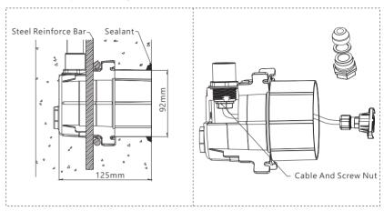
Insert the clamp ring into the niche before ceramic is applied. Wrap the power cord few round
