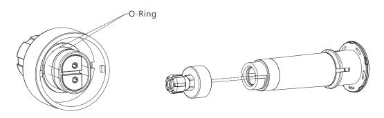
5) Wrap the cord and insert the light into conduit directly.
