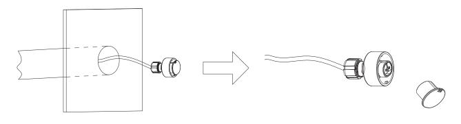
4) Make sure two O-ring are well assemble, then Connect the light and cord together and turn clockwise to lock.
