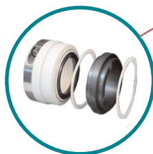
External type AISI-316L mechanical seal for highly corrosive fluids, static and rotating rings in SiC, spring and Polyester thermosetting powder coated power frame construction to prevent external corrosion
