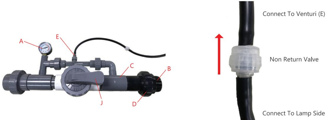
3. Screw the female hose fitting (E) onto the male thread of the Venturi circuit. The other end of the hose must be fitted into the elbow adapter, on the top of the system (F). There is a Non-Return valve (K) between (E) and (F) which is a one direction valve to prevent air go back to the UV lamp Ozone generator.
