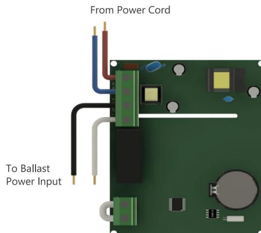
**NT-UV130TF** Timer version, remove the white color jumper and connect the flow switch red and black cable.
