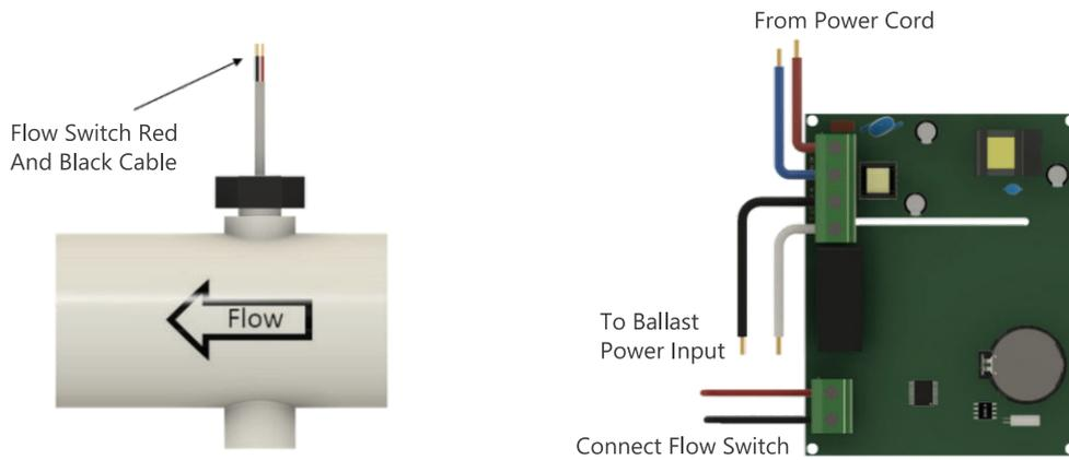
**NT-UV130F** without Timer version, there is flow switch controller PCB
