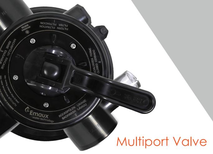
Emaux Valves are available in Top Mount and Side Mount design, constructed using ABS material with heavy duty plastic handle. The valves are characterized by 6 operating functions which cover all the necessary operations needed in any swimming pools filtration.
